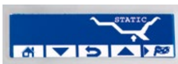
Programma moto statico e dinamico Bike program for static and dynamic balancing
